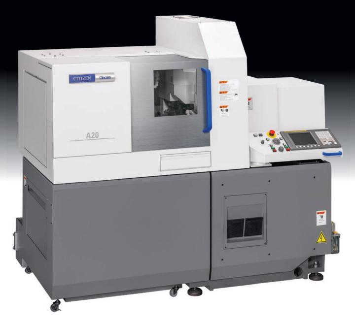
Acclaimed for its excellent cost to performance ratio, the A20 has evolved as a 5-axis machine for Ø20 mm applications with the advantage that it can be used with or without a guide bushing. Use as a regular guide bushing automatic lathe when machining long, slender workpieces or without a guide bushing for shorter parts with minimal bar end remnants. The guide bushing can be guickly and easily mounted and removed.
